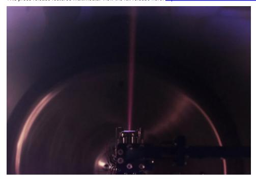
Momentus' Microwave Electrothermal Thruster (MET) undergoing ground testing in a vacuum chamber at company headquarters. Photo: Momentus.
